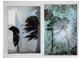
Left shows a standard window, right shows how ImpactGard® resists the impact from wind borne debris.
