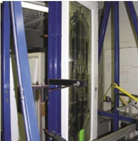
ODL Doorglass must survive our test of 50,000 slam cycles.
